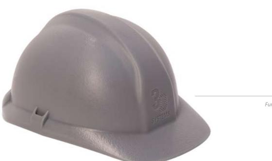
Functional prototype helmet used for durability testing
