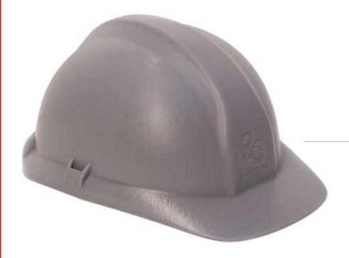
Functional prototype helmet used for durability testing
